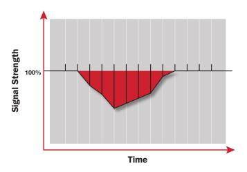
The level of emboli volume within the flowing blood will be dependent on the level of signal reduction multiplied by the number of signal reduction events.
