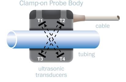
The transit time of the ultrasonic signal is decreased when traveling downstream with the blood flow and increased when traveling upstream against the blood flow. The phase delay between the integrated transit times is a measure of flowing blood.
